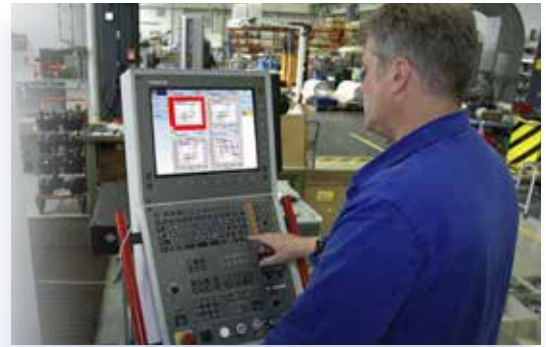
Process control and visualization directly on the machine control
