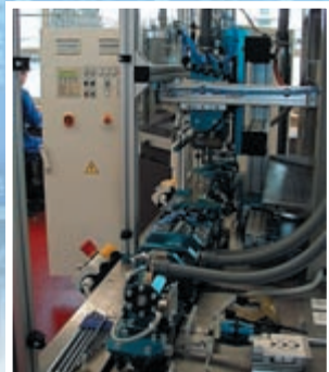
Functional test stand for inspection of finished products
