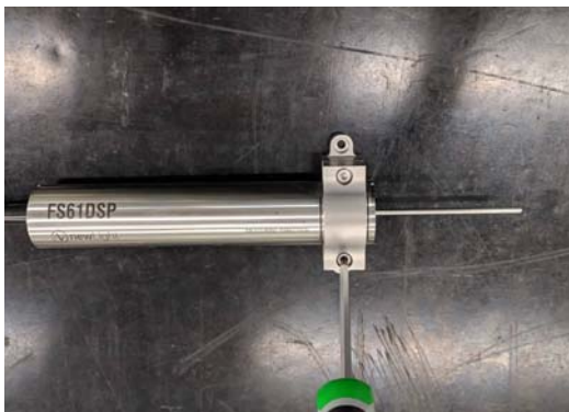
Fig. 2.5 Fixing the sensor brackets
