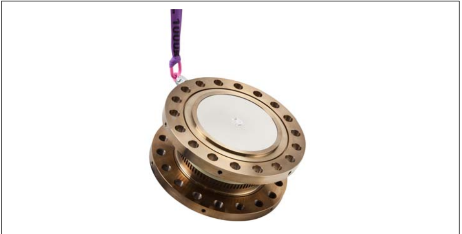
Fig. 5.3 Tilting the rotor
